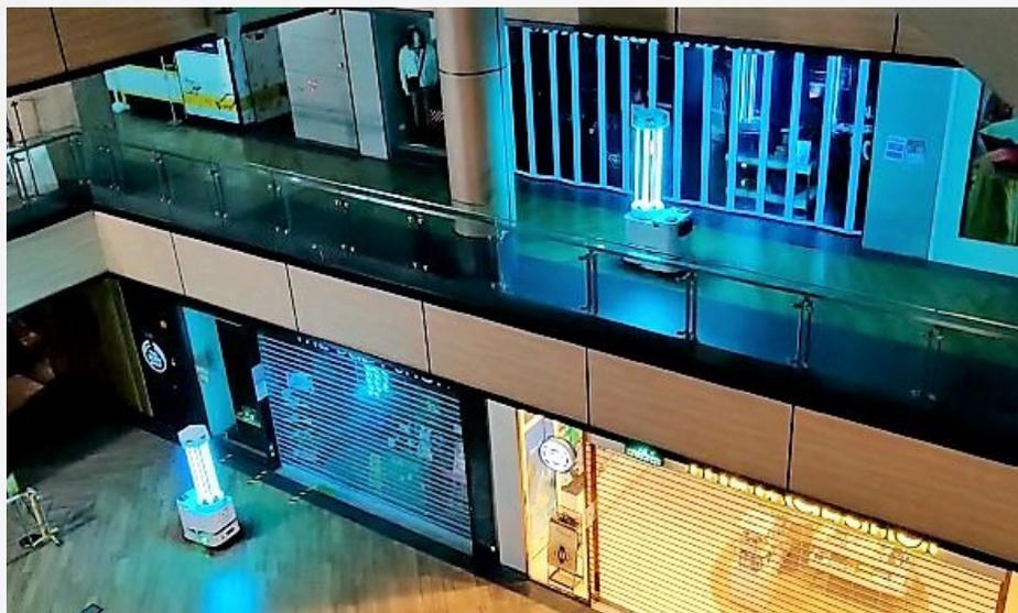
*PBA Sunburst UV-disinfecting autonomous mobile robot at Northpoint City, Singapore.
