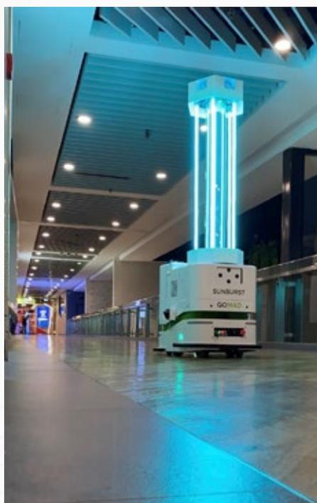
*PBA Sunburst UV-disinfecting autonomous mobile robot emits powerful UV-C rays which can eradicate viruses. [Photo credits to PBA Group and Frasers Property]*
